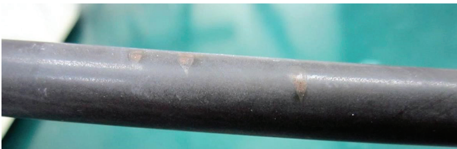
Biofilm formation due to improper cleaning technique
