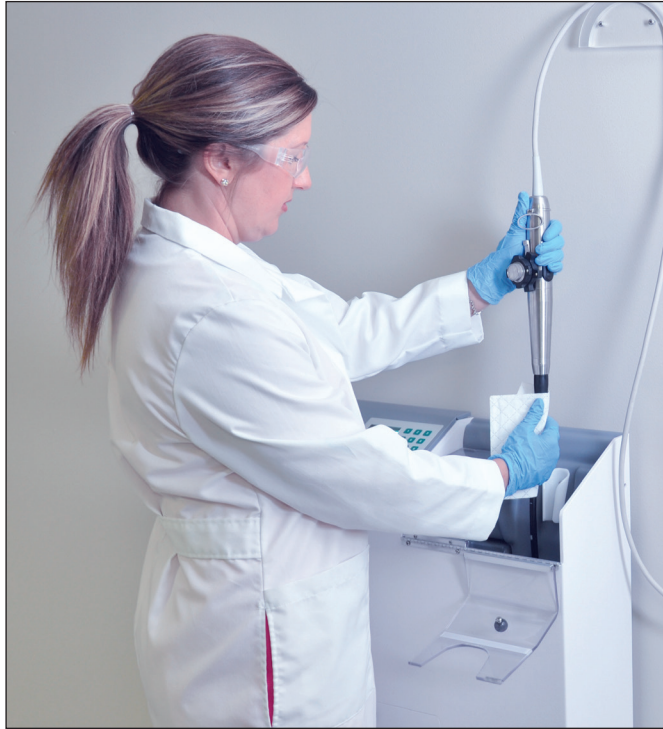
QwikDry® ultrasound drying cloth used in conjunction with CS Medical TD 100® and TEE ultrasound probe.
