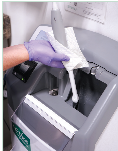
QwikDry used to dry a transvaginal probe after high-level disinfection and rinsing.
