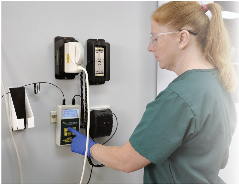
Electrical leakage testing of TEE probe
