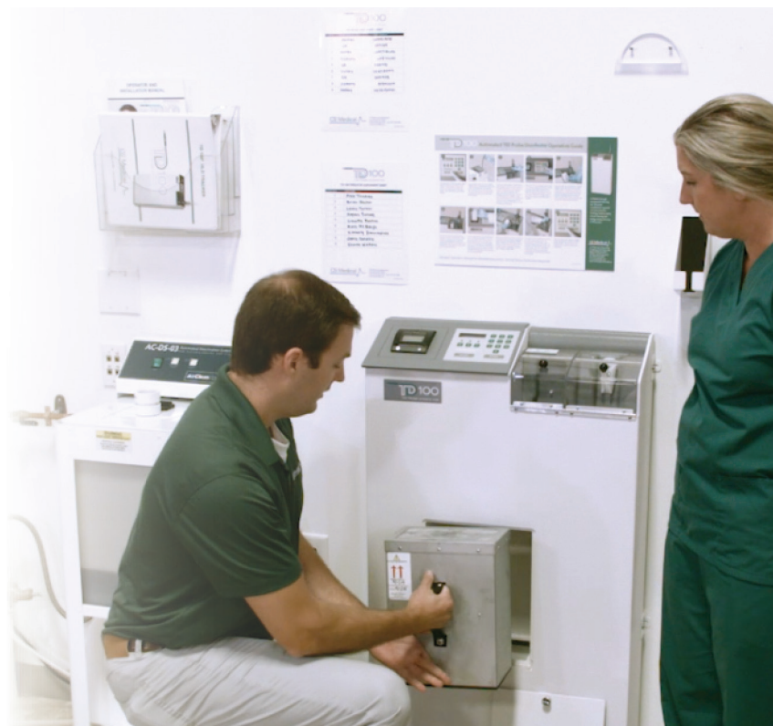
Vapor management filter for containment of HLD
