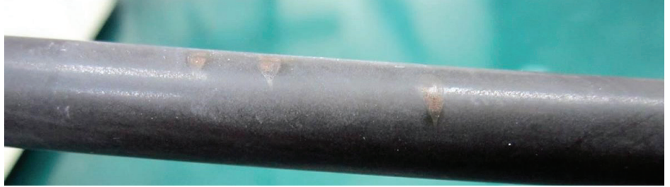
Biofilm formation due to improper cleaning technique.
