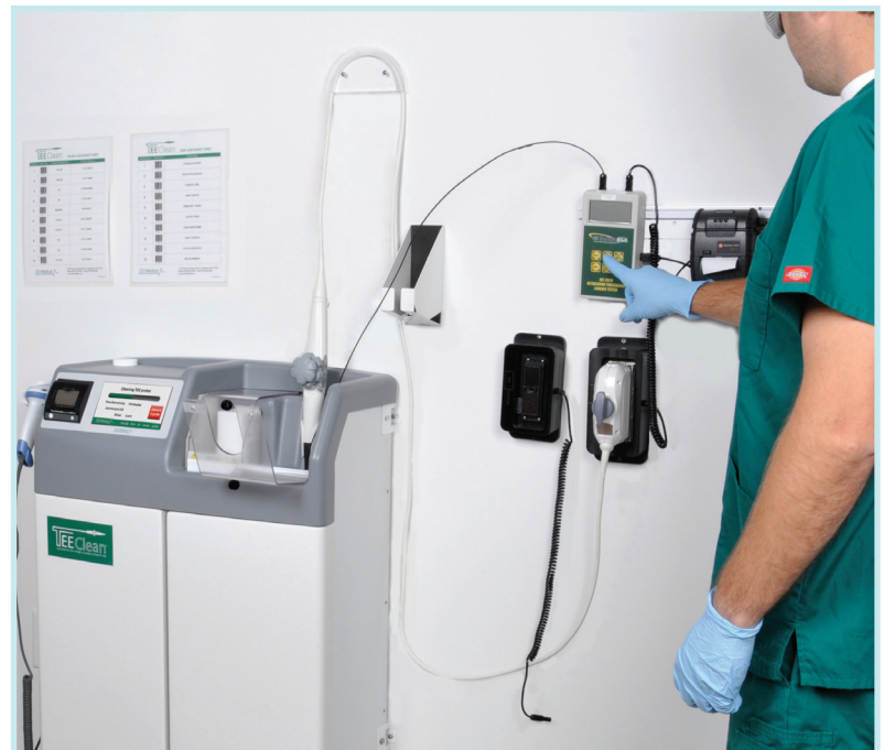
Electrical leakage testing can be performed while inside TEEClean
